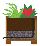
SuDS planters capture and manage roof runoff utilising rainwater to nourish plants while helping manage excess water. Rainwater is directed from the downpipe into the
