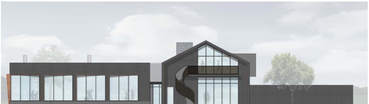
Figure 5: Revised West Elevation showing the introduction of a wall to close off the gable end to reinforce the barn typology, separate balcony and amended materials for balconies and external staircase
