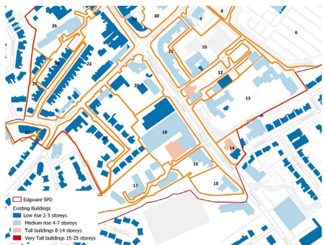
Figure 42 – Existing building heights (note the plan is derived from an analysis of heights in metres translated to storeys and therefore the number of storeys is indicative)
