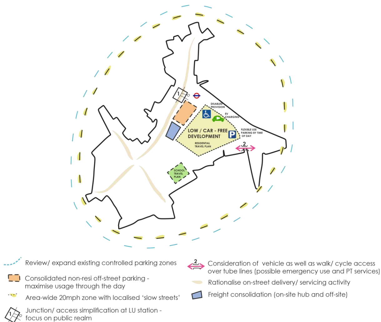
Figure 9 Schematic plan and descriptions of SPD highways measures
