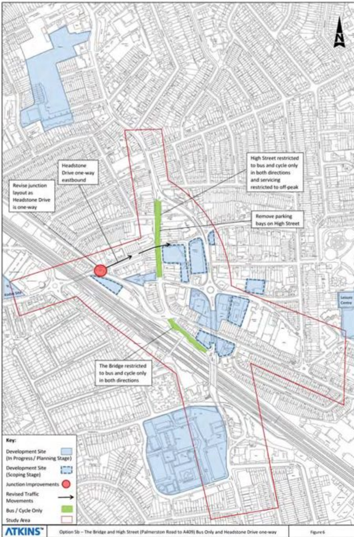
Figure 7-6 Option 5b – The Bridge and High Street (Palmerston Road to A409) Bus Only and Headstone Drive one-way
