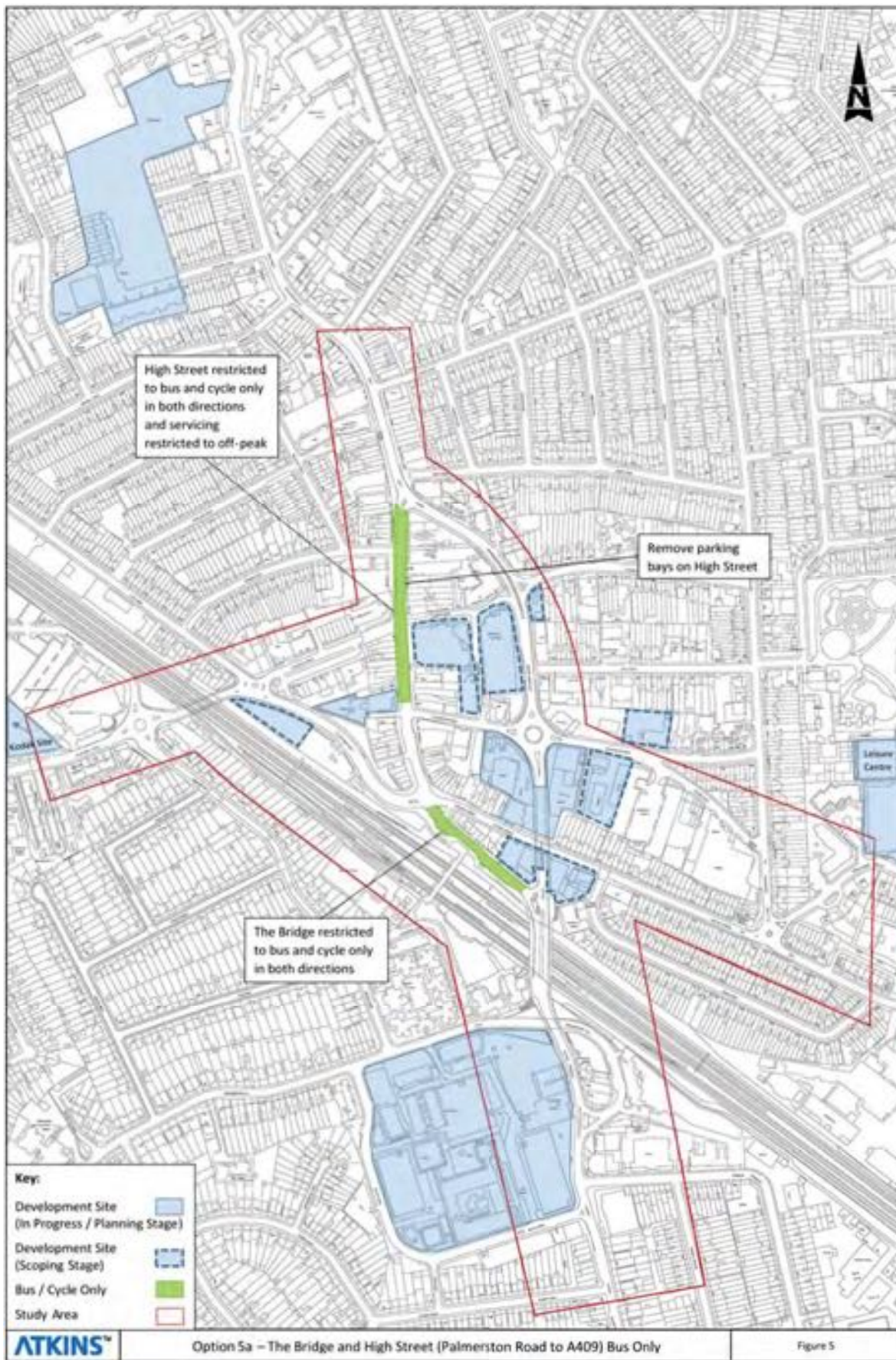
Figure 7-5 Option 5a – The Bridge and High Street (Palmerston Road to A409) Bus Only
