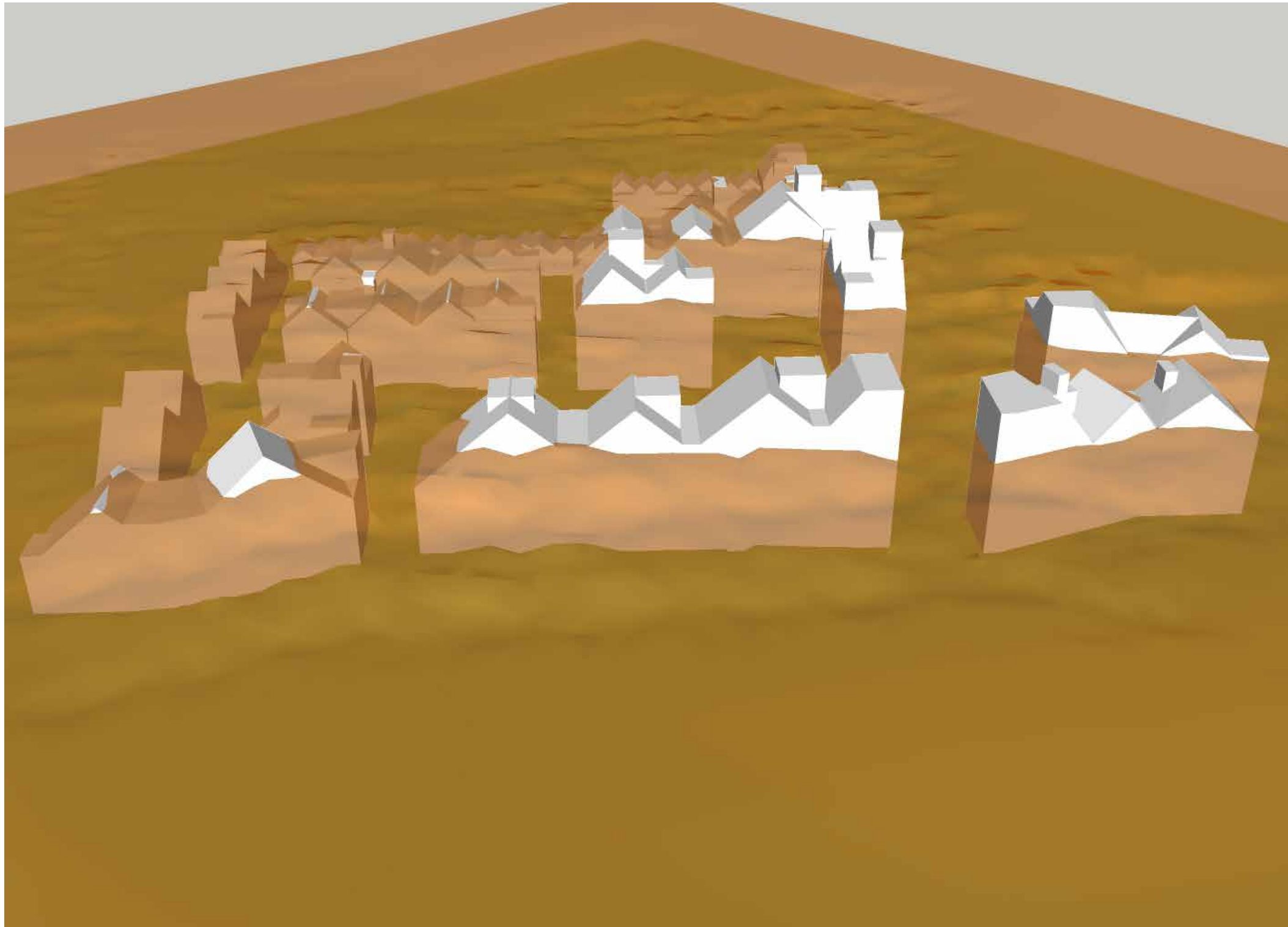
Maximum MOD Height Model; illustrating areas breaching the height restrictions
